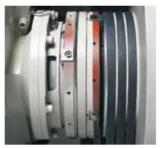
SHEAR BOLT (SAFETY BOLT)
