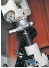
Should the knife strike a hard material, shear bolts are broken to avoid serious damage to the machine.
